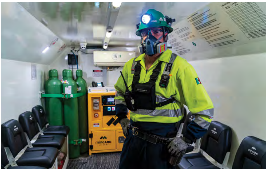
H&S Worker inspects the interior of the underground mine refuge chamber at the Juanicipio Project.
